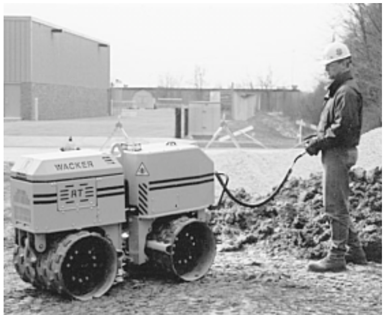
Figure 5-7 Walk-behind vibratory roller with remote control. (Courtesy of Wacker Corporation)
