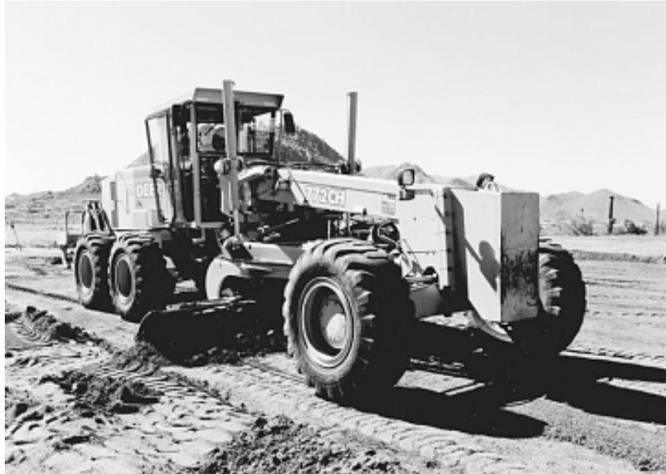
Figure 5-13 Modern motor grader. (Courtesy of John Deere Construction & Forestry Company)
