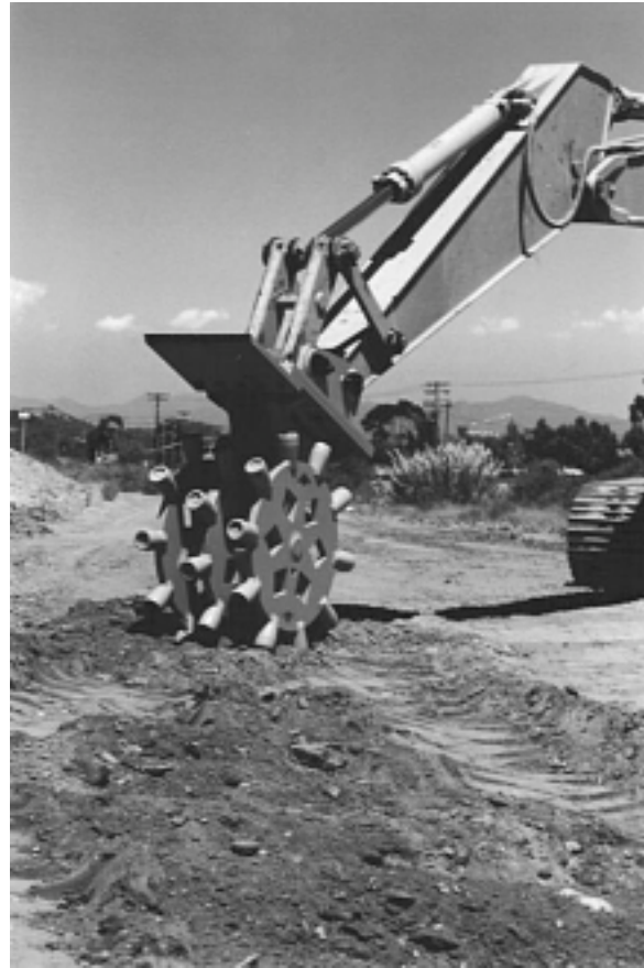
Figure 5-8 Compaction wheel mounted on hydraulic excavator. (Courtesy of American Compaction Equipment, Inc.)
