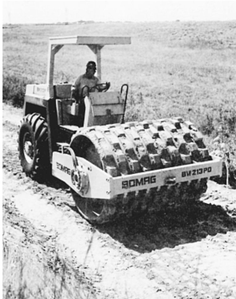
Figure 5-5 Vibratory tamping foot compactor. (Courtesy of BOMAG (USA))
