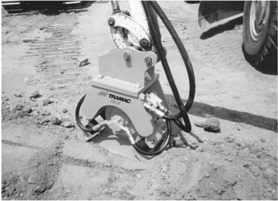
Figure 5-9 Vibratory plate compactor attachment for excavator. (Courtesy of Ingersoll-Rand Tramac)
